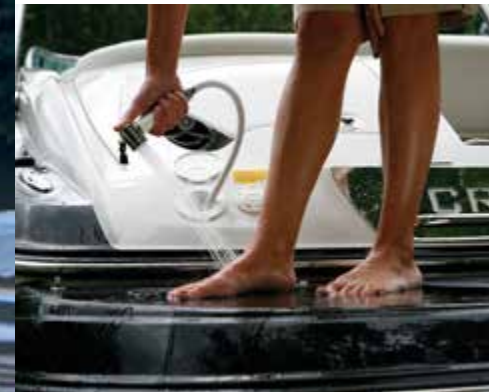
Optional transom with self-storing wash-down. Shown are stainless steel pull-up cleat and optional splash-proof stereo speaker.
