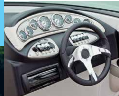
Optional black vinyl wrapped helm with Executive black steering wheel, Sony performance stereo and full instrumentation with stainless steel bezels.
